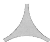
FIG. 3. (a) Network of Plateau borders of an open-cell aluminum foam [13]. The typical cell diameter is 6 mm. (b) Schematic of the cross section of a Plateau border channel through which liquid flows and whose cross-sectional area A is the basis of the foam drainage model.
